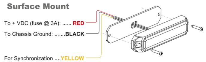
Connect YELLOW wires of all heads together for synchronization (all heads must be set at the same pattern)
